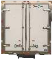
Drop "T" Handles : Trailer door gears made by S.S. material
