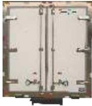
Drop "T" Handles : Trailer door gears made by S.S. material
